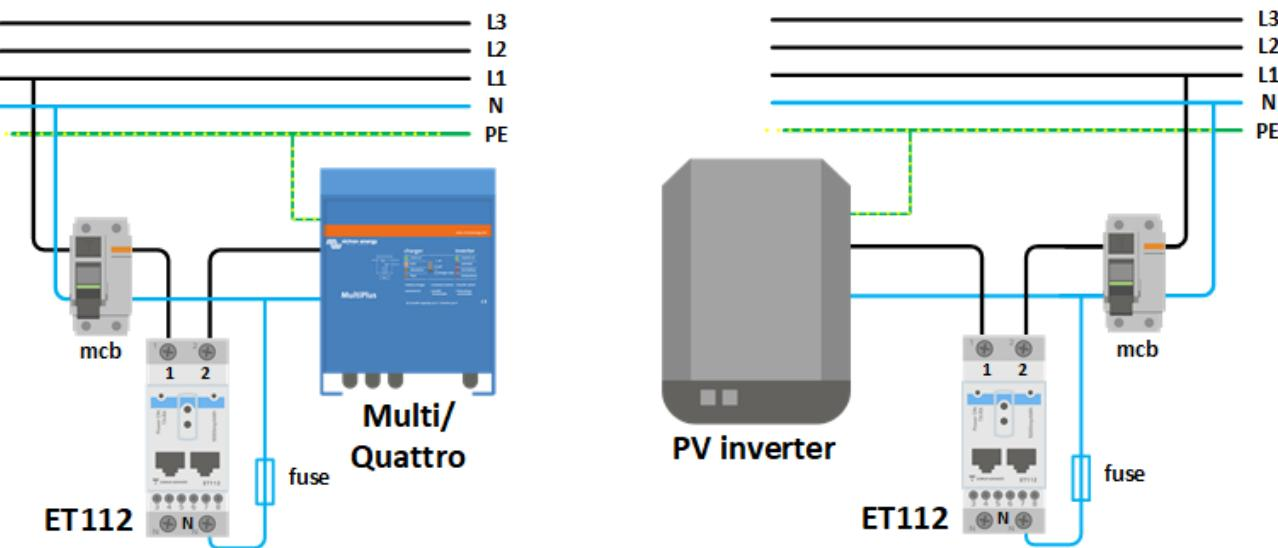
**Grid Meter** - Wiring when used as a grid meter. **PV Inverter** - Wiring when used to measure PV inverter or AC Genset.
