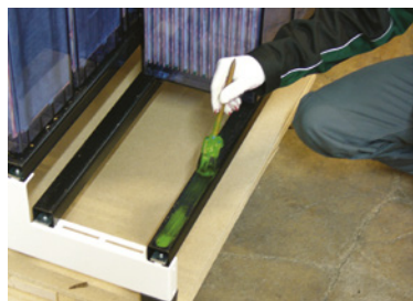
Fig. 5-13: Greased support profiles
