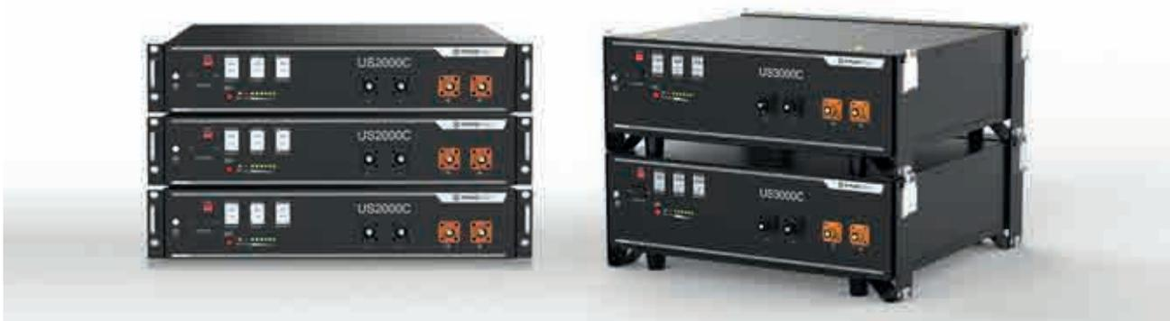
The storage modules comprise a lithium iron phosphate (LiFePo4) accumulator and an integrated battery management system (BMS) which constantly monitors the status of individual cells and these also provide protection against excessive levels of charge, voltage and temperature. This is how the BMS prevents an accumulator from failing prematurely as a result of ambient factors or operator error.
